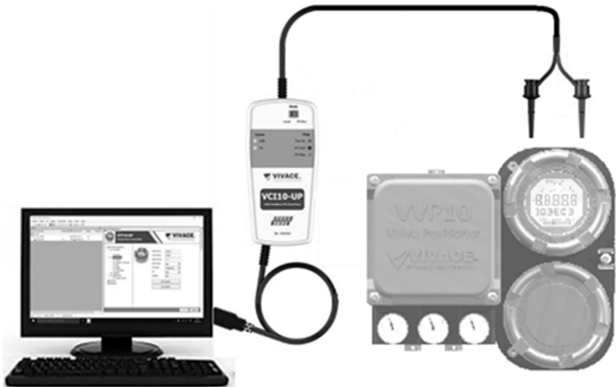
Figure 3.4 - Wiring diagram of VCI10-UP interface to VVP10-P.
